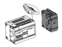
步骤 2. 将扩展模块对准主机接口推入到位后,反向推回锁扣进行扩展模块锁定。Then push the extension module into place against the mainframe interface and reverse the latch to lock the extension module.
